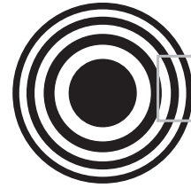
Figure 4: Michelson interferometer fringe pattern. What you are likely to see at first is a band of almost straight fringes, such as are shown within the grey box. What you then want to do is to adjust the tilt of M1 to get closer to the center of the fringe pattern, until at the end you get fringes that look like concentric rings as shown at right. Note that the center fringe can be bright, or it could be dark (it changes every time the net optical path length changes by \lambda/2 ).
