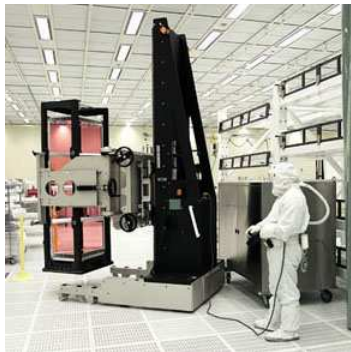
One replaceable amplifier slab on its mounting robot
